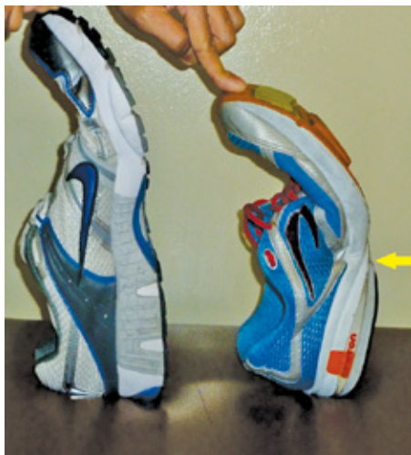
Figure 1. Shoe inspection revealed mechanical breakdown of the minimalist shoe's medial platform (right). The minimalist shoe (right) demonstrates a break in the midfoot, while the stability shoe (left) breaks at the metatarsal heads.
