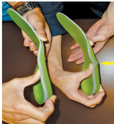
Figure 2. Comparison of the left orthotic used in the stability shoe (left) versus the minimalist shoe (right), clearly demonstrates a more dramatic breakdown of the minimalist orthotic at the medial arch.
