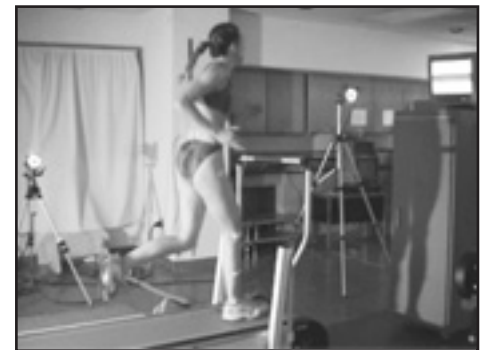
Figure 4. Subject running on the treadmill with retro-reflective markers placed on her pelvis, thighs, shanks, and feet. A video monitor (right) was provided for real-time feedback.
